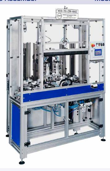
Full-automatic assembly unit, equipped with 2 modules for the automatic provision and assembly of internal sealing rings, bearing-tight and position-accurate.
